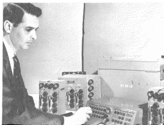
Figure 8—Comparison of microminiature translator (being adjusted) and the AN/AYA-1 .
