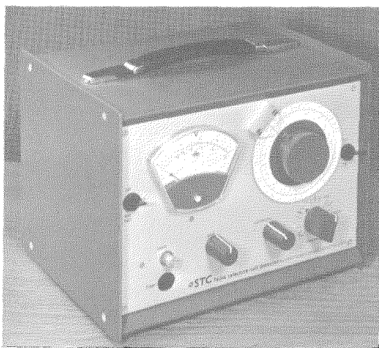
Figure 21—Selective null detector for bridge balancing and similar purposes.
