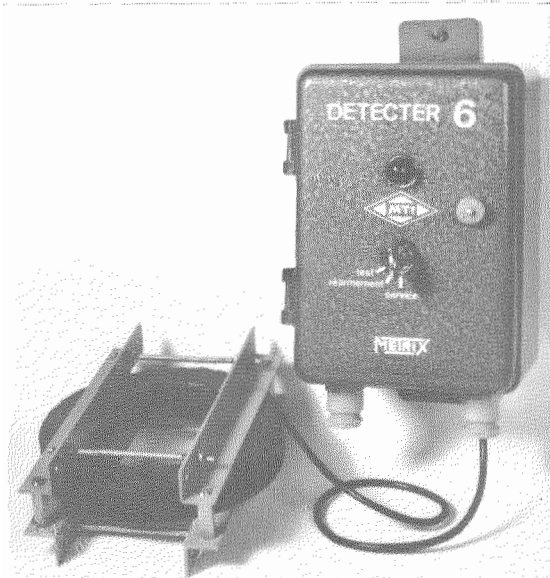
Figure 19—"Detector 6" for monitoring an electric circuit for leakage currents.
