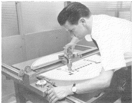
Figure 5—Artwork preparation on a coordinatograph.
