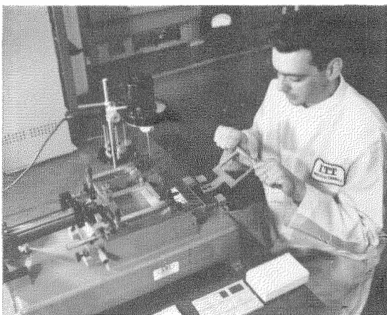
Figure 7—Semiautomatic screen printer, laboratory model.
